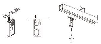
$\ensuremath{^{*}}$  Assisted installation tooling for fixing the stopper
